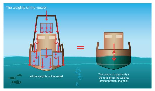
The total weight of the vessel, including all the stores, fuel, equipment and fishing gear, can be represented as acting through one point—the centre of gravity (G).
