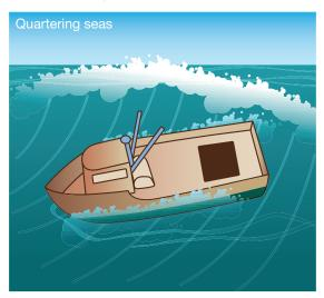
Quartering seas are even more prone to broaches, wave attack and swamping than following seas. On every wave, the vessel is partially broached on the wave face, increasing the chances of a full broach. The quarter is exposed to breaking waves and the deck exposed to swamping.
