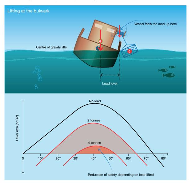
How much the stability safety is reduced, depends on the load lifted and whether a derrick is being used.
