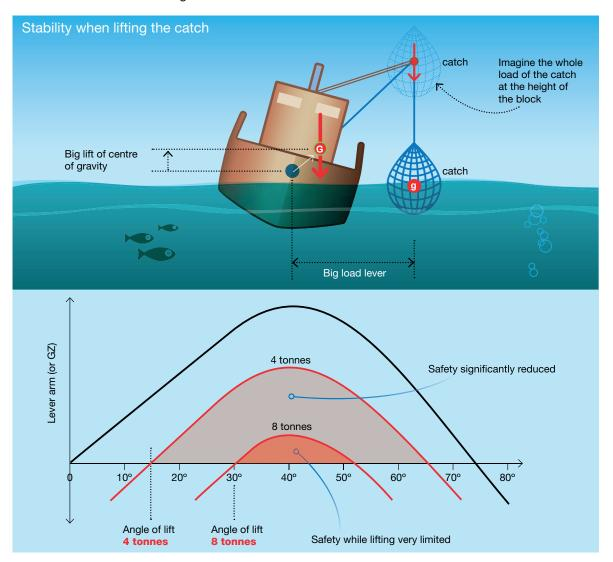
Lifting fishing gear or a catch out of the sea into the air shifts the full weight to the highest point of the wire, usually just above the blocks on a derrick or A-frame. This sudden jump in the vessel's centre of gravity can be very dangerous. By the time you notice the vessel feels 'soft', it may be too late!
