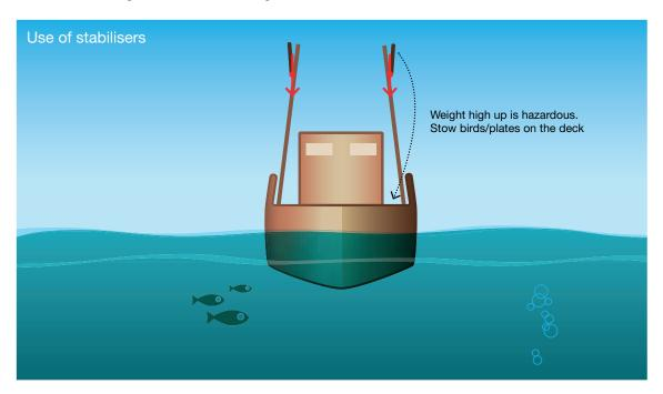
The plates, lifting surfaces or 'birds' must always be stowed on deck while they are not in use. They can weigh more than 100 kg, and leaving them at the top of the arms will significantly reduce a vessel's stability.
