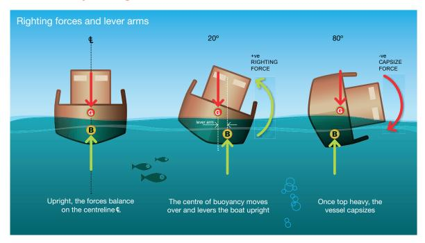
Upright in flat water, the forces at G and B balance each other on the centreline of the vessel.
