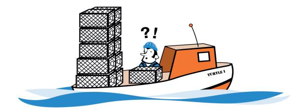
If you have a stability book, look at the 'loading conditions' prepared for your vessel. Loading conditions have been calculated for your vessel for specific amounts of fuel, stores and catch. Each scenario is designed to help you plan your trip and to highlight when the quantities of catch and/or fuel become a hazard. They should be thought of as useful guides to help you operate your vessel safely.
