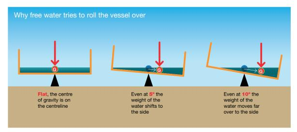
The diagram shows how the free-surface effect tries to roll the vessel over. It applies to water on deck, fuel and ballast in tanks, bilge water and melted ice in the fish holds.
