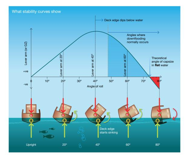
The graph shown above is a stability curve, sometimes called a righting-lever curve or a GZ curve. You will find some of these for your vessel in your stability book if you have one. The small vessels that sit underneath the graph illustrate the corresponding angles of roll and how the forces acting on the vessel move.
