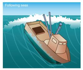
trying to turn the vessel. At the same time, the rudder often has a loss of control due to the motion of the following wave and being raised near the surface as the stern lifts.
