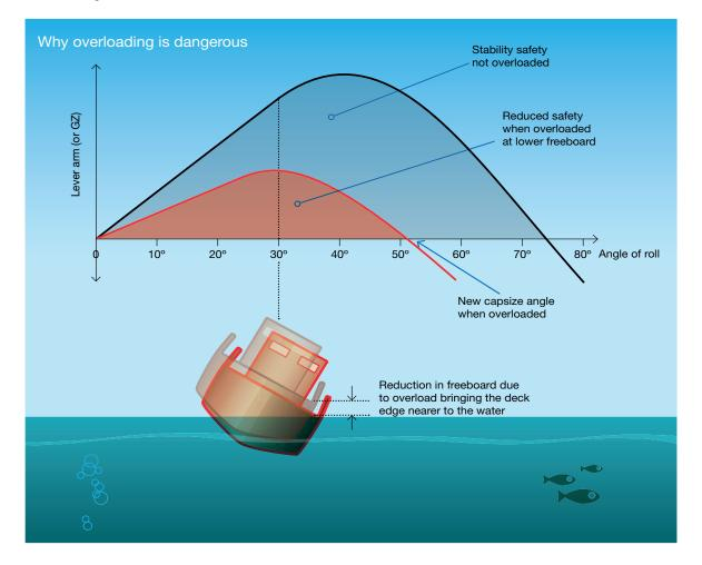
Loading too much catch on the deck has two significant negative effects. Firstly, it overloads the vessel (as described) and reduces the freeboard (and range of stability). Secondly, it lifts the average of all the weight on board (lifts the centre of gravity) and makes the vessel more top heavy. This combined effect is important to remember, as it can be dangerous and needs to be guarded against.
